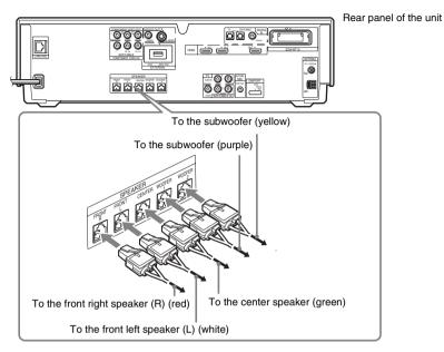
The speaker cords (yellow and purple) are connected to the subwoofer beforehand as follows. When re-connecting, be sure to match the speaker cords to the appropriate terminals on the speakers: the speaker cord with the color tube to  $\bigoplus$ , and the speaker cord without the color tube to  $\bigoplus$ . Do not catch the speaker cord insulation in the speaker terminals.
